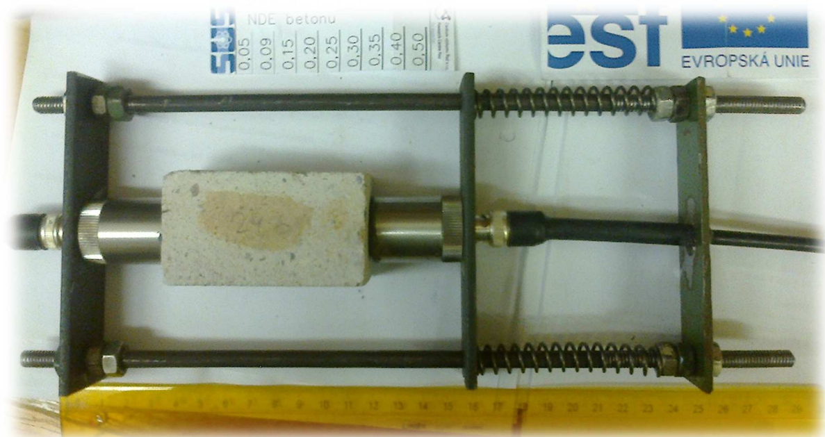
Figure 3. Special steel holder of ultrasonic transducers capable to the hot cells for concrete samples testing
