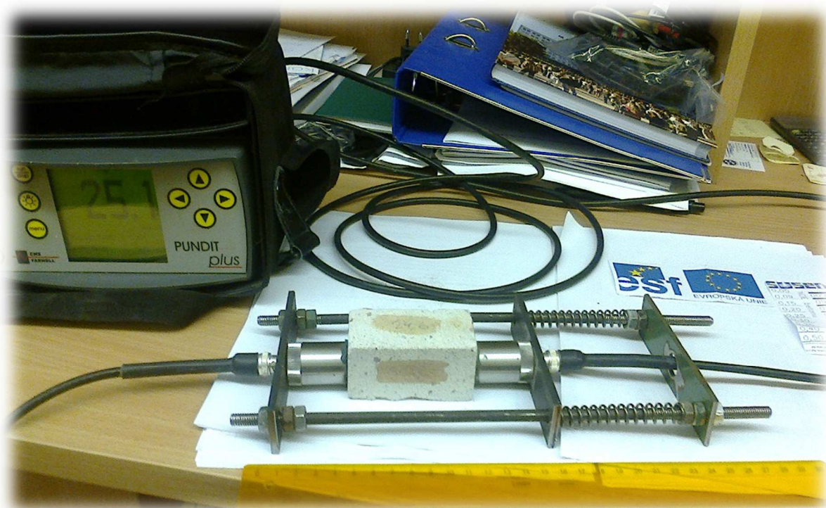
Figure 4. Testing of special steel holder function by ultrasonic instrument PUNDIT plus.
